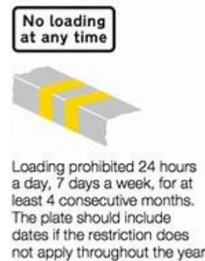
Figure 1 Example of yellow lines and signage
